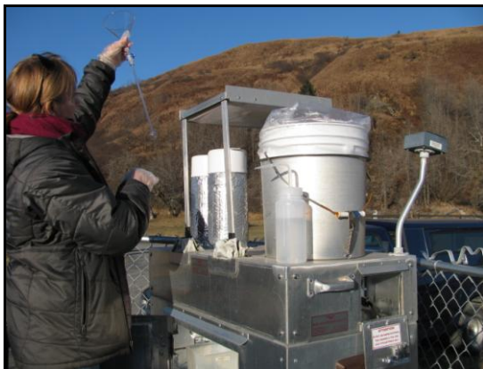
Barbara Trost, DEC, removes glassware while demonstrating mercury monitoring sample collection techniques (left). The monitoring site at the Kodiak Fairgrounds after a snow storm, KSWCD has an agreement with DEC to manage this station (right).
