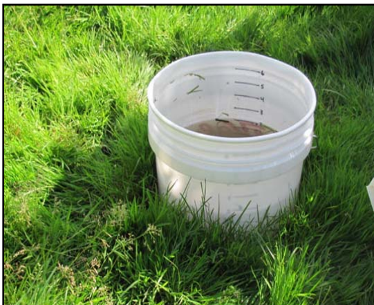
A bucket with the bottom cut out is used for percolation tests to help design rain gardens. Perc rate is used to help determine the depth of the rain garden and soil amendments to use.
