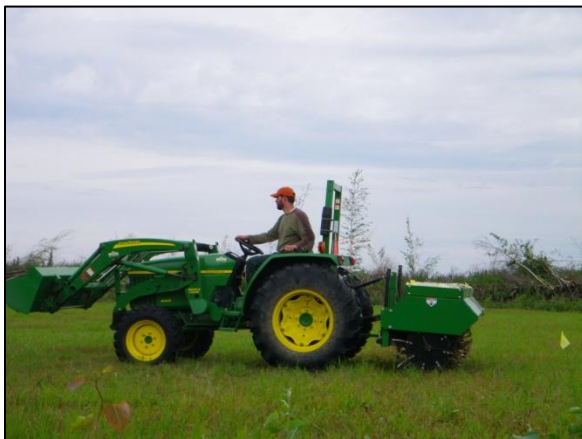
George Hitz using the soil aerator to improve soil quality and plant health in a hay field.
